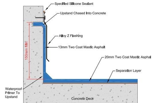
CAST CONCRETE UPSTAND DETAIL
