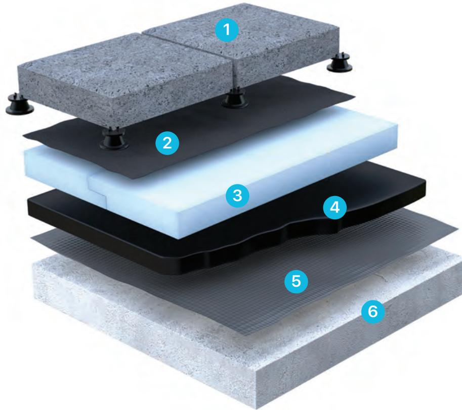
1. 40mm Paver or tile on a tile jack. 88.8 kg/m<sup>2</sup>
