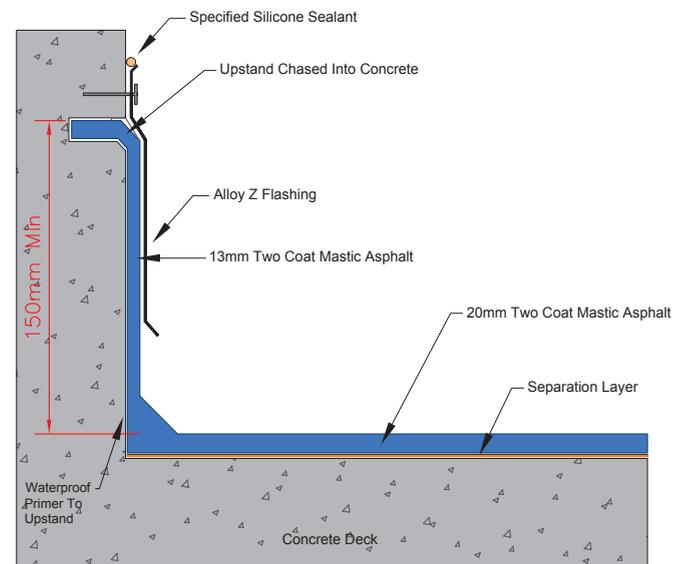
*Cast concrete up stand detail*
