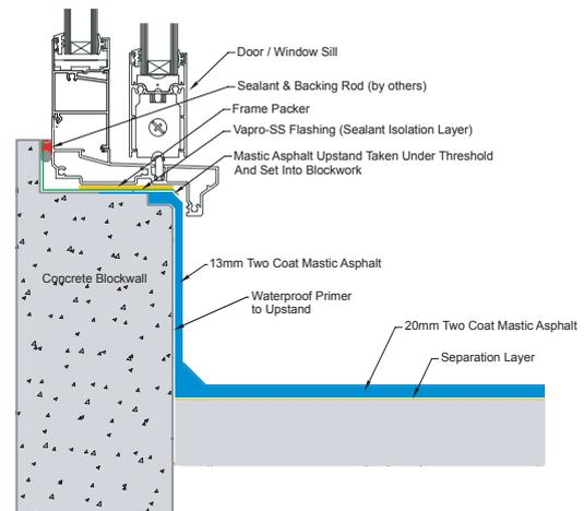
BLOCKWALL THRESHOLD UPSTAND DETAIL
