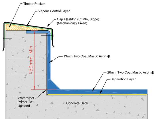
CAST CONCRETE PARAPET WITH CAP FLASHING
