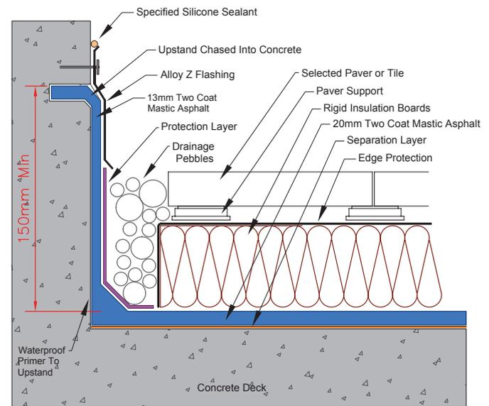
*Neuchâtel Mastic Asphalt inverted insulated roof X-sectional*
