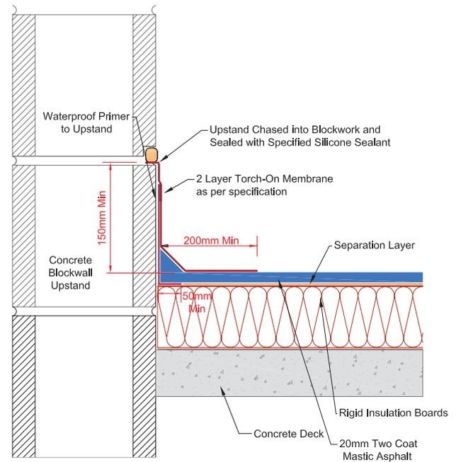
*Neuchâtel Mastic Asphalt insulated car park - roof X-sectional detail*
